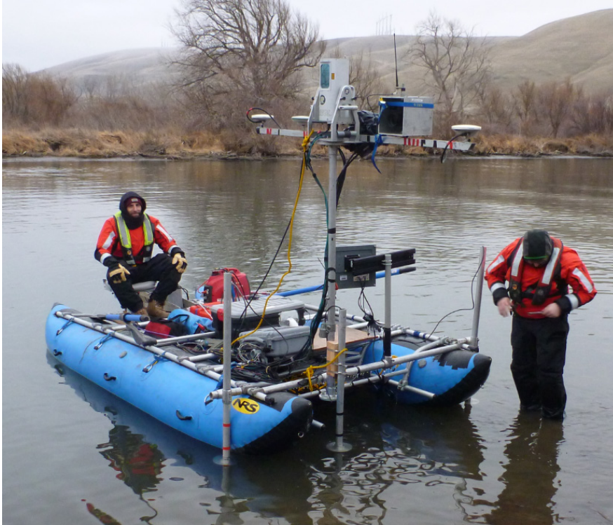
Figure 2-1. Tetra Tech Survey Vessel (R/V Screaming Seagull ) with vessel-mounted LiDAR and sweep system in deployed position
