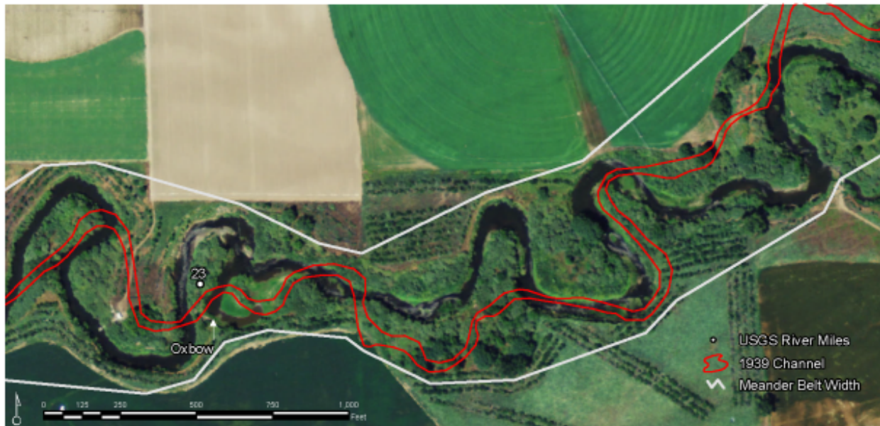
Figure 3-11. Example 2013 Aerial Photograph and 1939 Mapped Channel Location within Geomorphic Reach 6 Showing Channel Meander Pattern and Progression and Approximate Belt Width (the photograph shows an example cutoff and oxbow)
